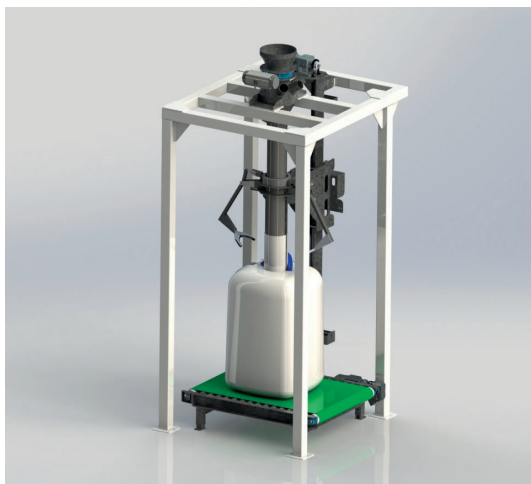
Brutto system without weighing hopper
